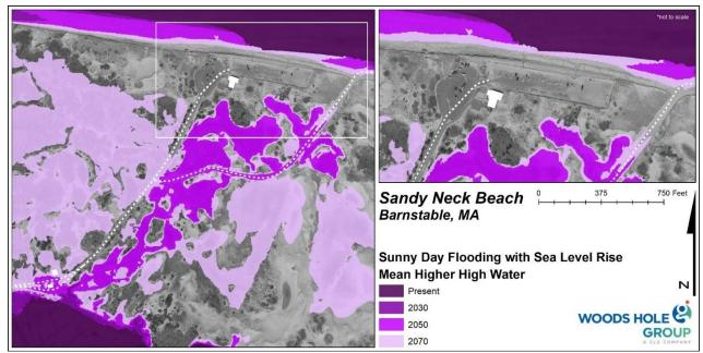
Figure 10. Projected flooding during MHHW during present day, 2030, 2050, and, 2070 time horizons.
