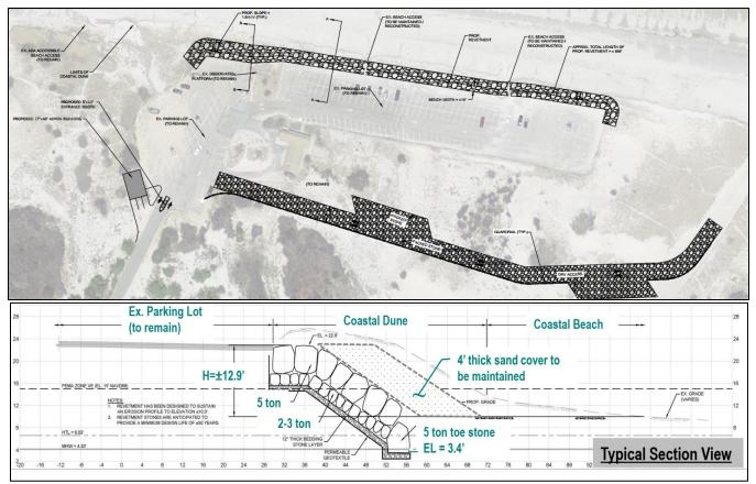
Figure 11. Plan view (top) and cross-section (bottom) of conceptual Alternative #2 from the 2016 study.
