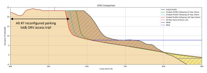
Figure 22. XBeach storm simulations for Alternative #7 with predicted 2050 sea level showing initial and eroded profiles for Transect #2.
