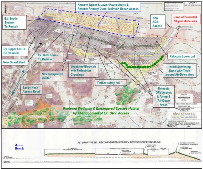
Figure 17. Plan view (top) and cross-section (bottom) of conceptual Alternative #5D from the 2016 study.
