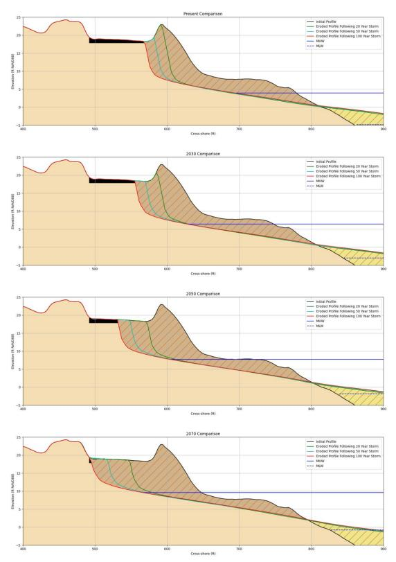
Figure 5. XBeach storm simulations at Transect 2 for present day conditions (top), 2030, 2050, and 2070 (bottom).
