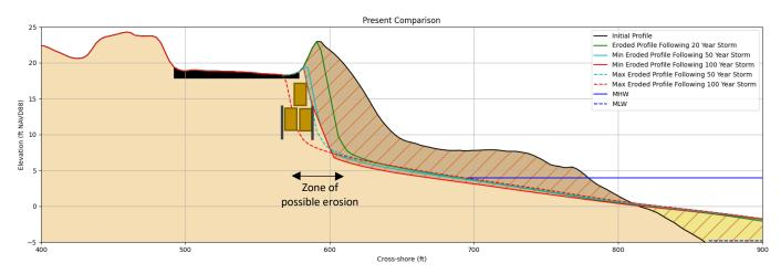
Figure 15. XBeach storm simulations for modified Alternative 3 with present day sea level showing initial and eroded profiles at Transect 2.
