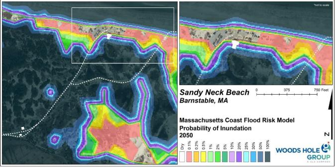
Figure 8. MC-FRM probabilities of inundation for projected sea levels in 2050.
