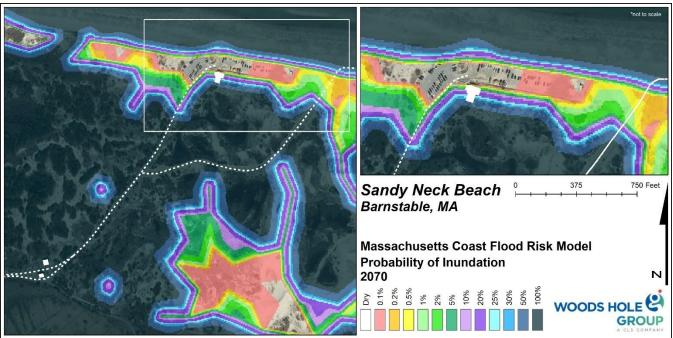
Figure 9. MC-FRM probabilities of inundation for projected sea levels in 2070.
