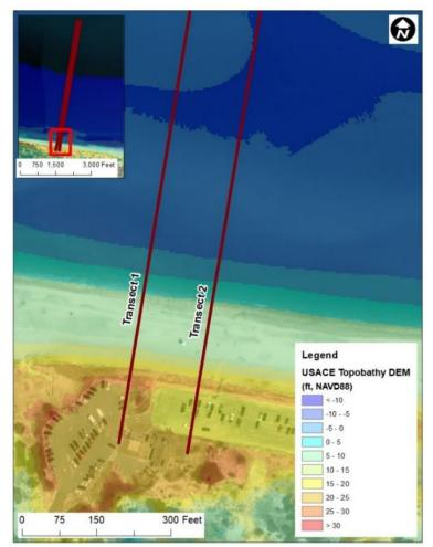
Figure 4. Transect locations used with the XBeach model and topobathymetry at Sandy Neck Beach Park.
