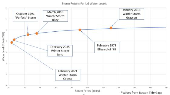
Figure 3. Return periods for water levels produced by past storms impacting the Sandy Neck Beach Park area.
