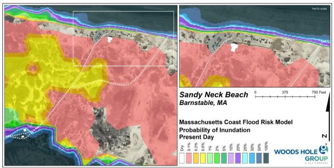
Figure 6. MC-FRM probabilities of inundation for present day sea level.
