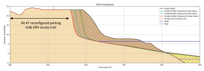
Figure 21. XBeach storm simulations for Alternative #7 with predicted 2030 sea level showing initial and eroded profiles for Transect #2.
