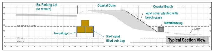
Figure 14. Cross-section of modified Alternative #3.
