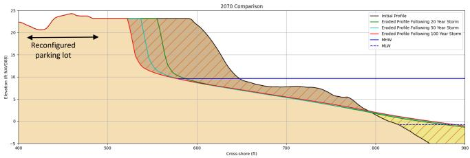
Figure 18. XBeach storm simulations for Alternatives #5A through #5D with predicted 2070 sea level showing initial and eroded profiles for Transect #2.
