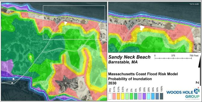
Figure 7. MC-FRM probabilities of inundation for projected sea levels in 2030.
