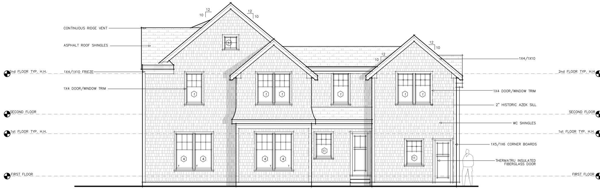
**PROPOSED REAR/WEST ELEVATION**
